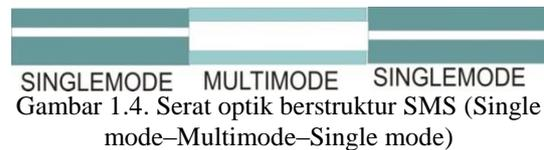
Gambar 1.4. Serat optik berstruktur SMS (Single mode–Multimode–Single mode)
