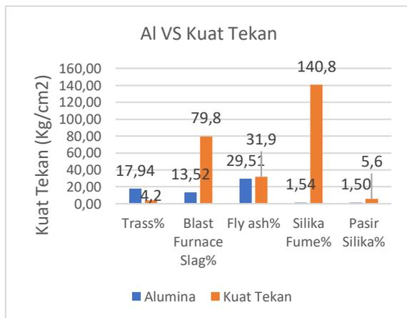
**Gambar 2.** Kandungan Alumina VS Kuat Tekan (Uji XRF)
