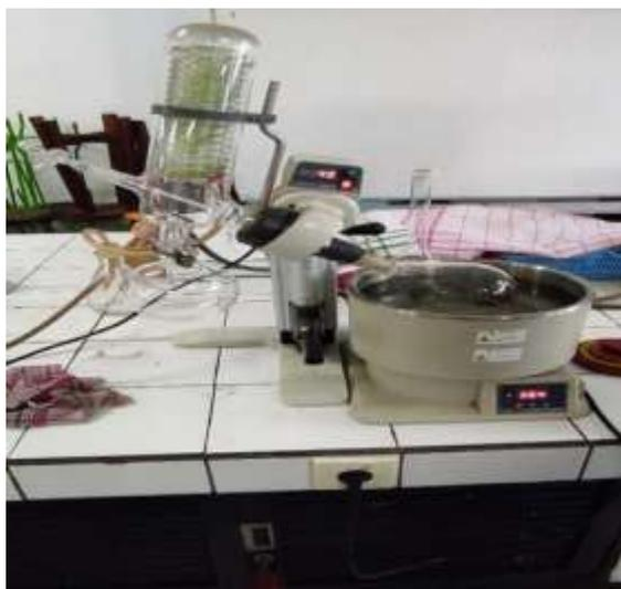
Gambar 9 - Rangkaian Alat Rotary Evaporator
